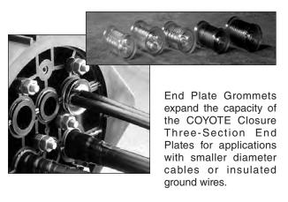
The grommets are manufactured from a weather-resistant urethane material that is designed to ensure a tight and permanent seal. A Silicone Sealant is provided to lubricate the grommet and cables for easy installation.
