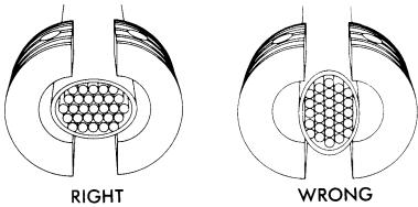
Using the cable shaper, compress cable to form a slight oval. Then, place End Plates as shown.
