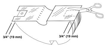
Apply LOCK-TAPE™ Sealant to End Plate halves without stretching. Leave 3/4" (19 mm) of sealant extending beyond End Plate on both sides. Square cut the tape way from bolt holes.
