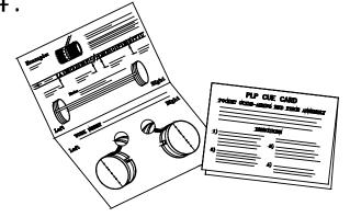
Use the PLP® CUE CARD as a worksheet to assure correct cutter blade size, proper hole cutting locations, and correct amount of LOCK-TAPE Sealant.
