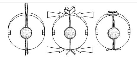
Using a ratchet wrench, draw the End Plate halves together evenly until the excess LOCK-TAPE™ Sealant separates and lays back.
