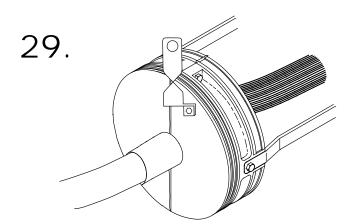
For Aerial Applications attach Aerial Hanger Bracket (available from PLP) to Insert on exterior of both End Plates, and attach to strand with messenger clamp (not provided).
