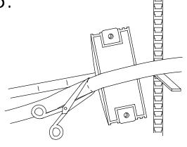
Use the Torque bar assembly to mark area to be cleaned and scuffed. Mark a 6" (152 mm) cable opening and coat scuffed area with C-Cement and allow it to dry to a tacky base.
