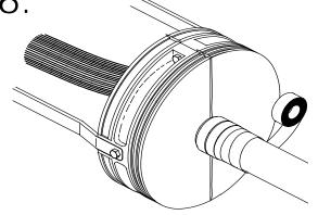
Apply two wraps of vinyl tape over exposed LOCK-TAPE™ Sealant on cables.
