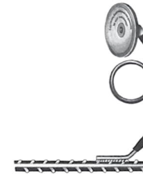
Earthing Bond on Ribbar
